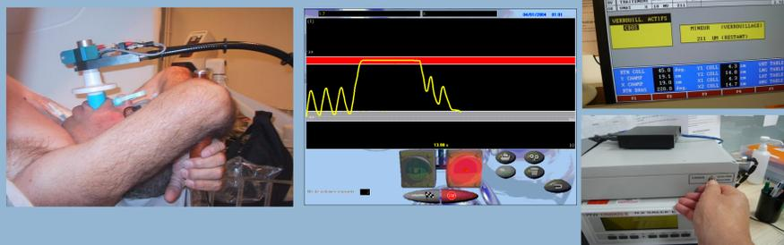
A phantom plan, two QA plans and two patient plans were used to voluntarily test interruptions during the irradiations. To evaluate the potential impact of breath hold interruptions, we used the Delta4™/Scandidos system and MLC Dynalog files records.
